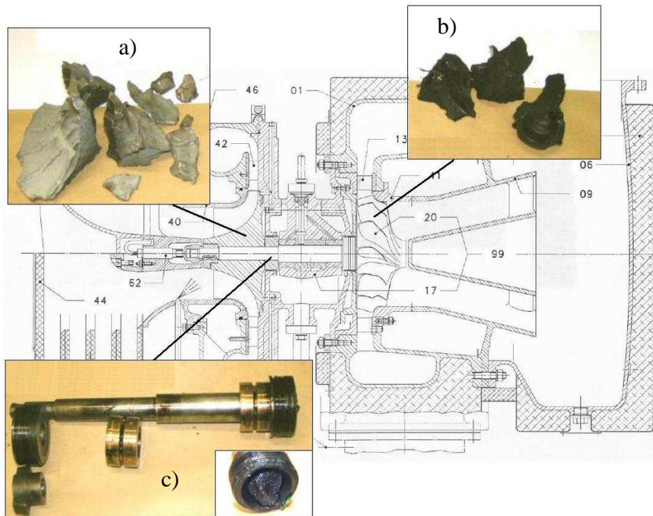
Fig. 1. Rest of the turbocharger working elements after the failure: a) – compressor rotor, b) – turbine rotor, c) – propeller shaft, bearings, and labyrinth sealing
