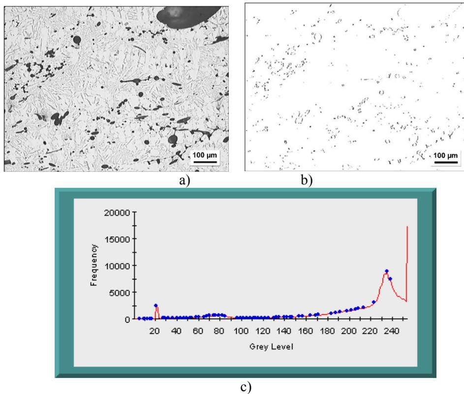
Fig. 2.3. A trial computer-aided analysis of a porosity image (Aphelion software); material:  $\text{Al}_2\text{O}_3/\text{SiO}_2$  fibre, AlSi matrix (non-etched specimens); a – output image [1], b – unsuccessful attempt [1], c – grey level histogram.
