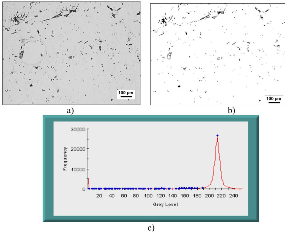
Fig. 2.4. A trial computer-aided analysis of a porosity image (Aphelion software); material:  $\text{Al}_2\text{O}_3/\text{SiO}_2$  fibre, AlSi matrix (silver-sprayed sample), area of  $225\times$ ; a – output image, b – unsuccessful attempt, c – grey level histogram.
