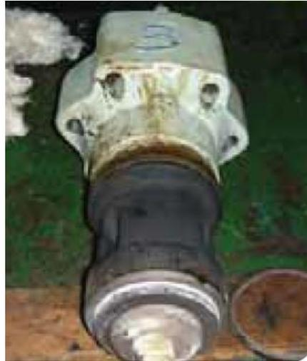
**Figure 3.** Photograph of the starting valve removed from the engine after an explosion in the starting air manifold (Royal Belgian Institute of Marine Engineers 2009).
