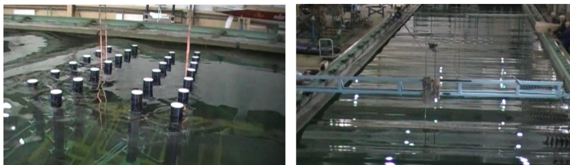
Figure 8. The damping device in the course of tests in the model basin of the Ship Hydromechanics Division, Ship Design and Research Centre (CTO S. A.) in Gdańsk.
