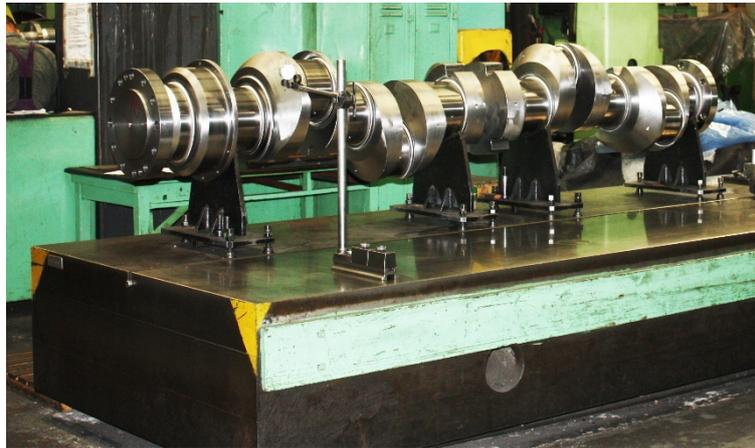
**Figure 5.** Measuring station for crankshafts for medium-speed engines.
