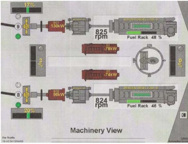
Figure 2. Power and propulsion system of UT 755 hull design vessel.
