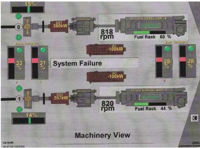
Figure 3. Power and propulsion system of UT 755L hull design vessel.
