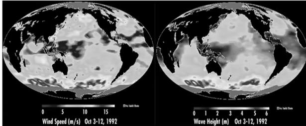
Fig. 1. Global wind speeds and wave heights correlation [6]
