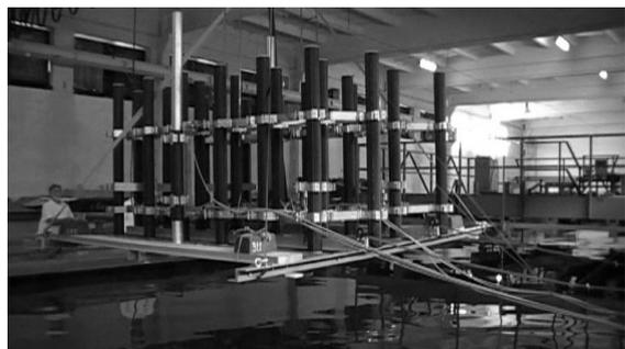
Fig. 9. Testing the submarine breakwater prototype in the towing tank of the Ship Hydromechanics Division, Ship Design and Research Center SA, Gdańsk, Poland [22]
