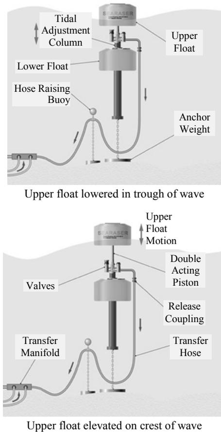
Fig. 4. The floating system *Searaser* of *Ecotricity* [5]
