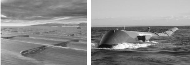
Fig. 6. Attenuators of *Pelamis* [16]
